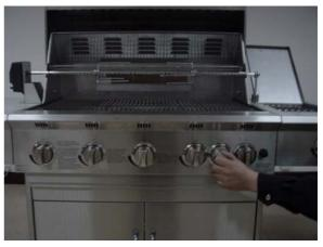
3.After the rotisserie burner is lit, adjust the knob as desired.
